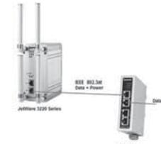
PoE Injector. Then the AP can be powered and user can access its management interface through the cable. The figure on the right is an example of Connect AP to the PoE injector. **Note:** Please choose Korenix Industrial IEEE 802.3at compliant PoE Injector or Switch as power input source. Thus Korenix can provide better quality assurance for your network.
